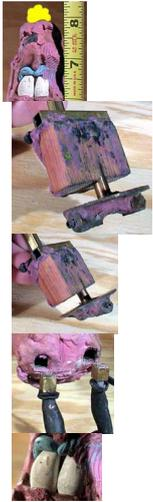
One thing we learned was that they used 1/2 inch hex cap head machine screws to secure the puppets to the set floors. They would first drill a hole in the wood floor, and screw the hex screw down to pull down on the feet. You can see on the top left why this would save a puppet from getting ruined using a phillips head wood screw and screw driver. The allen wrench on the top right is angled away from the puppet, and when you turn it you wont hit the sculpted areas.
